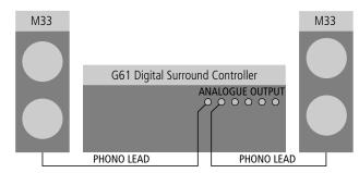
• Connect the appropriate analogue out sockets from the digital surround controller to the speaker inputs, using phono leads.
