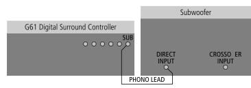
Connect the SUB analogue output socket from the G61 Digital Surround Controller to the subwoofer's line-level input using a phono lead.
